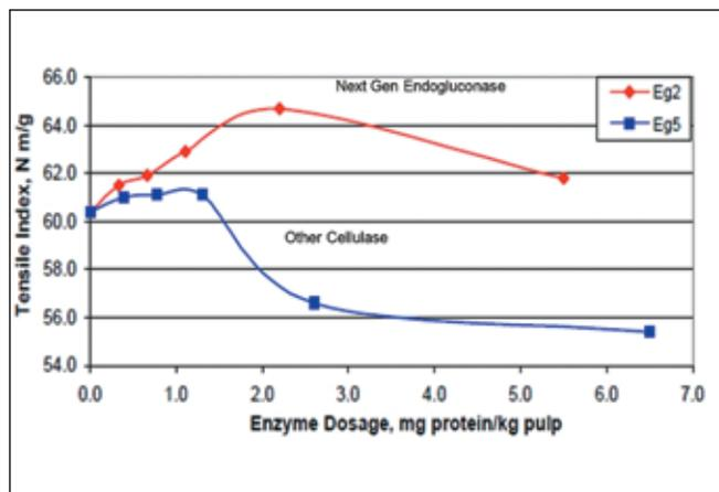
Figure 3. Enzyme dosage vs. Tensile Strength (BSWK).
