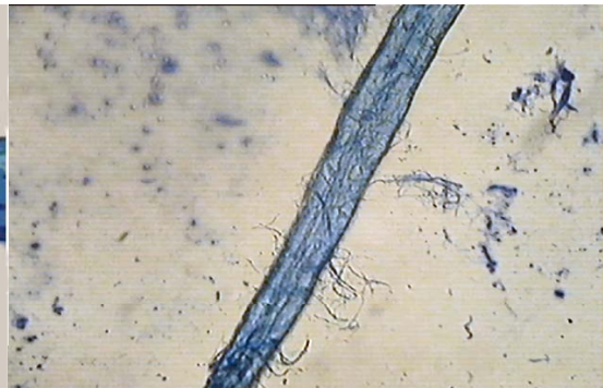
Fig. 2b. Softwood Control With PFI Treatment.
